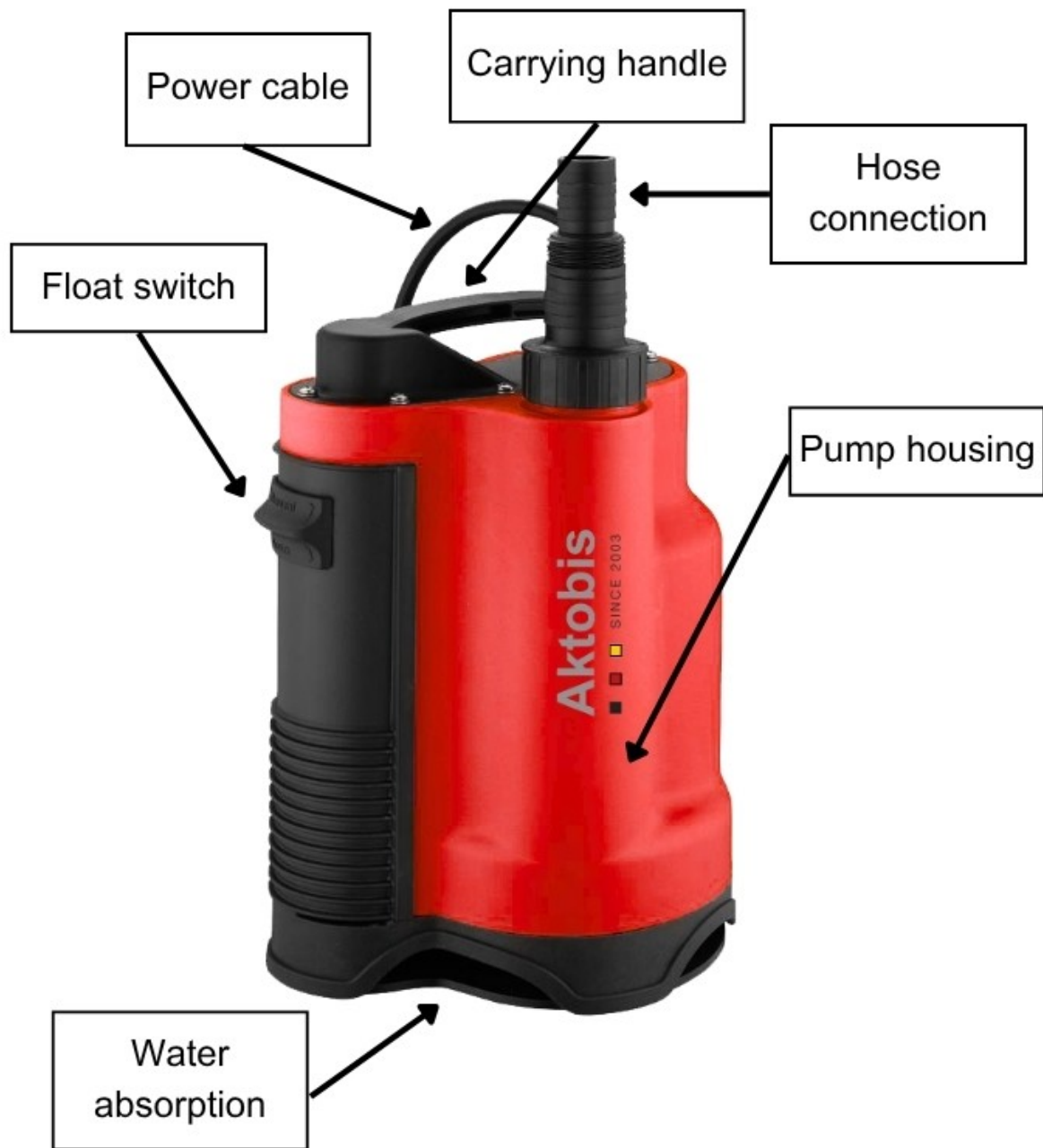
Fig. 1: WDH-SP750 Submersible Water Pump – main components.
